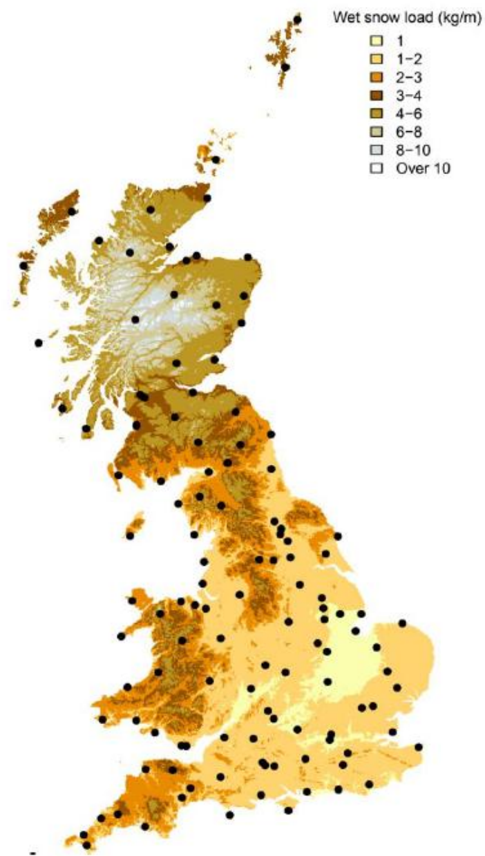
Figure 2-10: Estimated wet snow load in Britain with 50-year return period interpolated to a regular grid of 500m resolution by regression kriging. Black dots: Locations of the weather stations used in the analysis.
